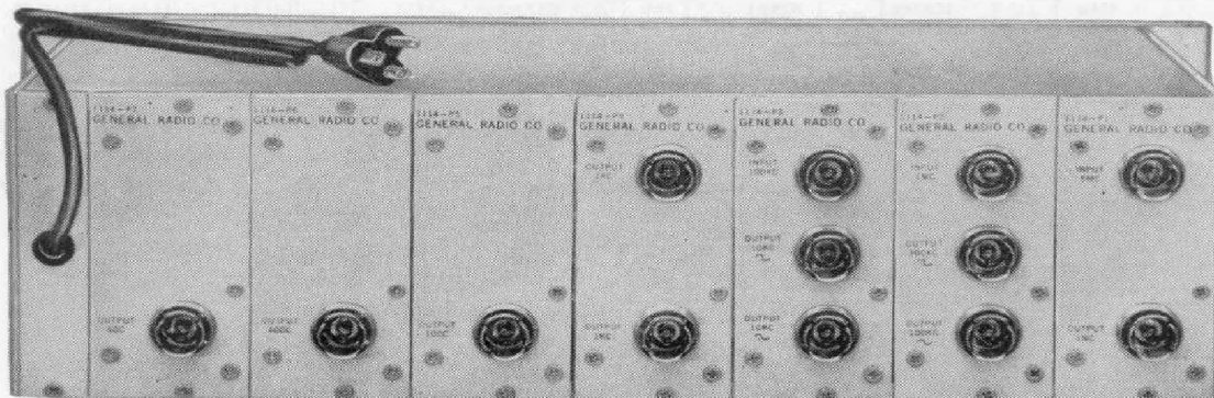
Figure 8. Rear view of the divider with plug-in units installed.
