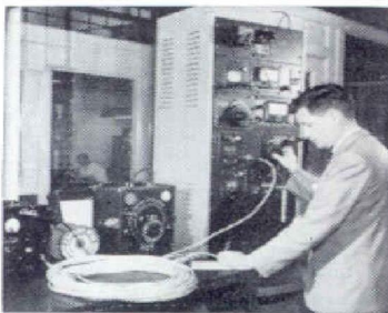
Richard L. Brereton, of Canada Wire and Cable Co., Ltd., Leaside, Ontario, well-known authority on cable testing, is shown operating his convenient, rack-mounted assembly of General Radio equipment for the measurement of attenuation and other characteristics of high-frequency cable.
