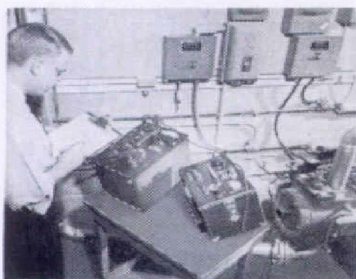
The Type 1554-A Sound and Vibration Analyzer with the Type 761-A Vibration Meter, as set up for the measurements on an air compressor (see Figure 4, page 5).
