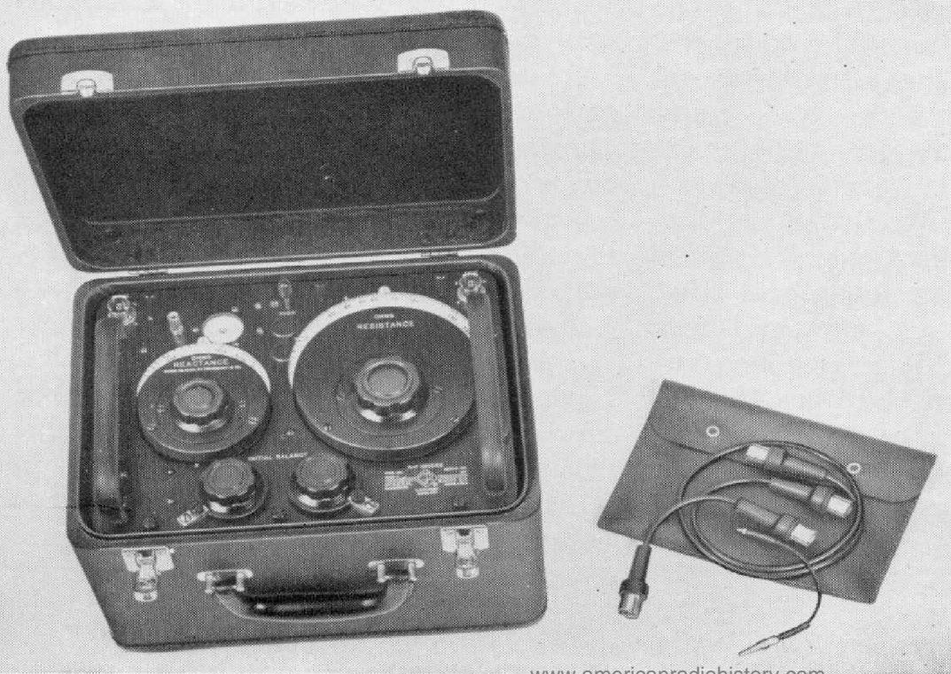
Figure 1. View of the Type 1606-A Radio-Frequency Bridge in its carrying case. Shielding is provided by the metal cabinet of the instrument, so that the bridge can be used either in or out of the carrying case.
