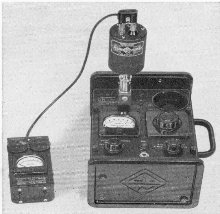
Figure 1. View of the Type 1552-B Sound-Level Calibrator, installed on the Type 1551-A Sound-Level Meter and driven by the Type 1307-A Transistor Oscillator.
