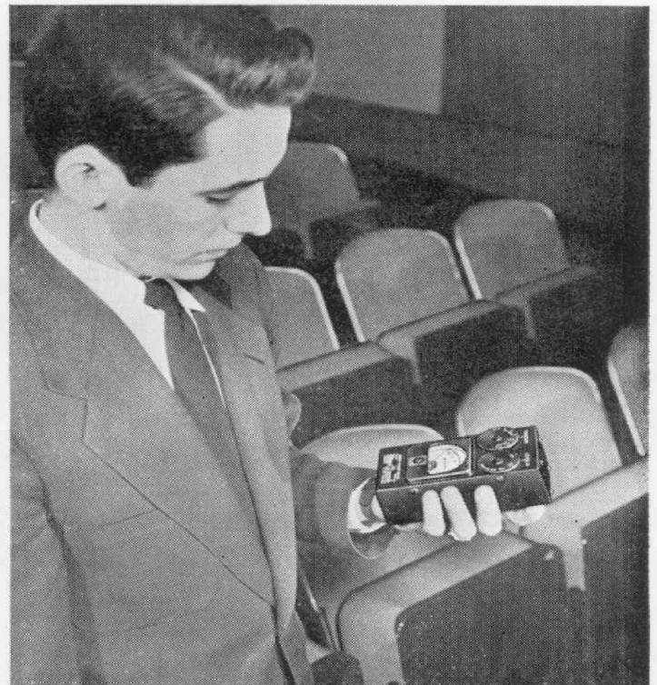
Figure 8. Measuring the level of reproduced sound in a theatre.
