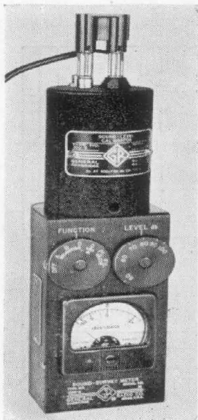
(Right) Figure 7. Sound-Survey Meter being used to measure noise level produced by pneumatic rock drills.
