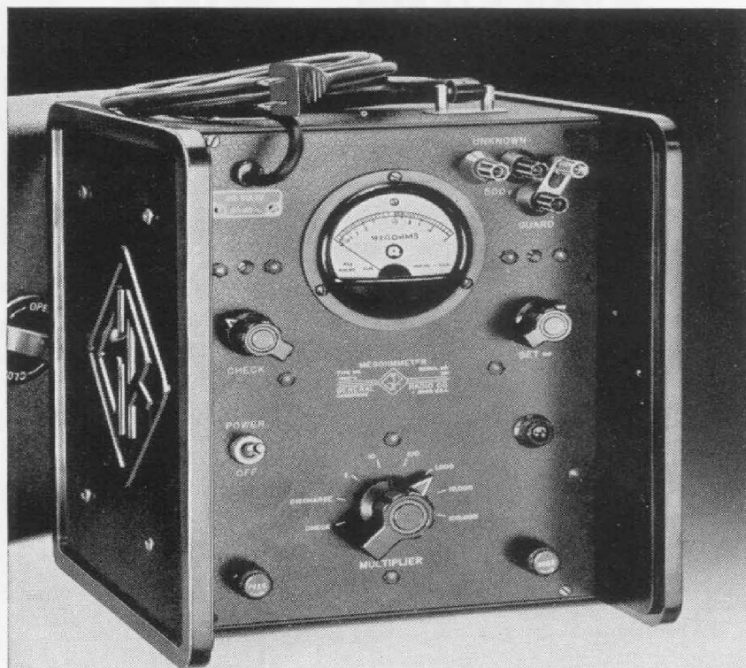
Figure 1. View of the megohmmeter with cover removed to show panel.
