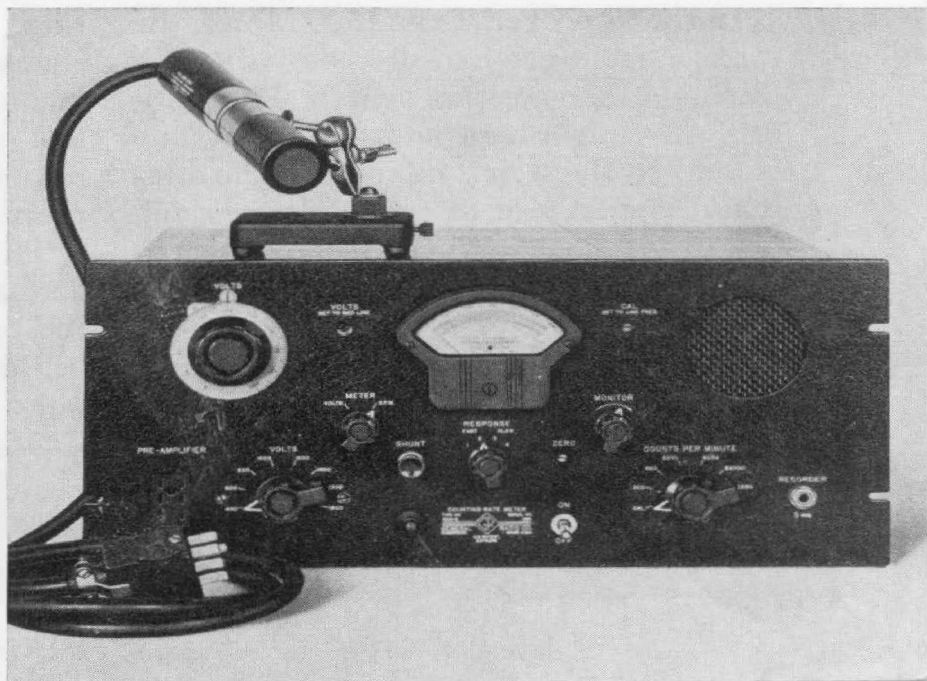
Figure 1. Panel view of Type 1500-B Counting-Rate Meter with counter tube and probe stand.
