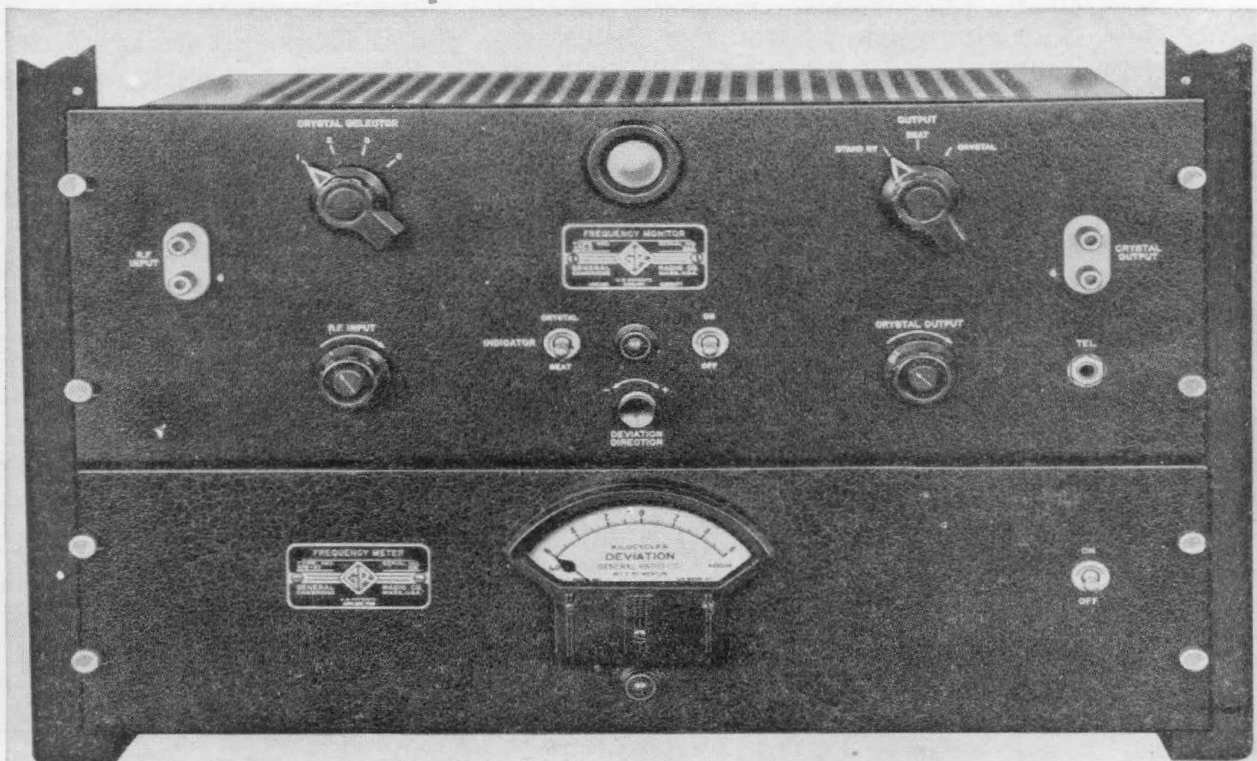
Figure 1. Panel view of the complete video frequency monitor.
