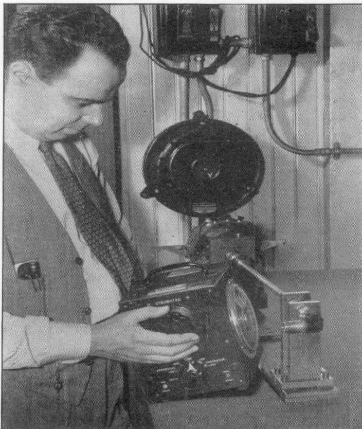
FIGURE 1. Mr. Frank Wilkins of the Barbour-Stockwell Company reading the relative positions of the drum dials by means of the Strobotac.
