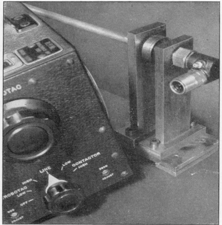
FIGURE 2. Close-up of the torque meter. The two drum dials, one carrying an index, the other a scale, are shown between the two vertical supports.
