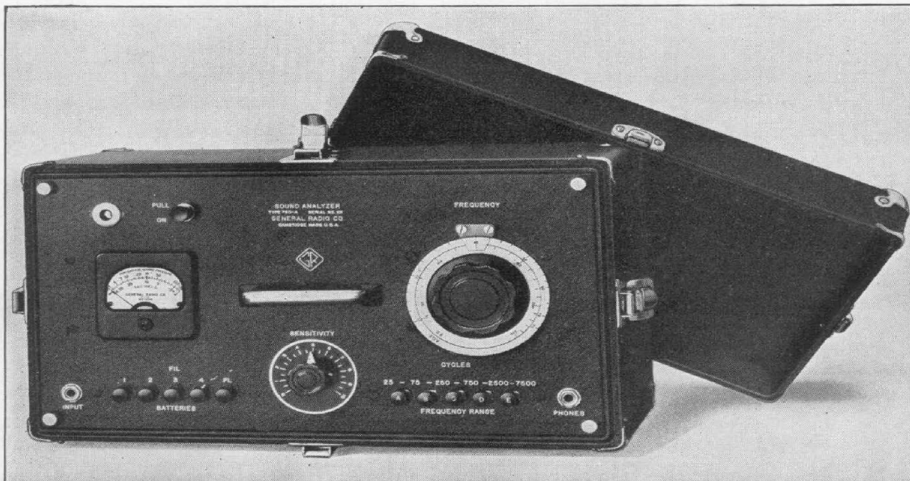
FIGURE 12. View of the TYPE 760-A Sound Analyzer with cover removed.
