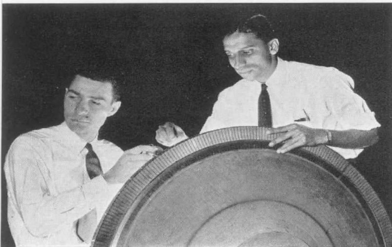
FIGURE 3 (above). Engineers move the crystal pickup along the bucket tips. The pickup output is fed to the cathode-ray oscillograph shown below.
