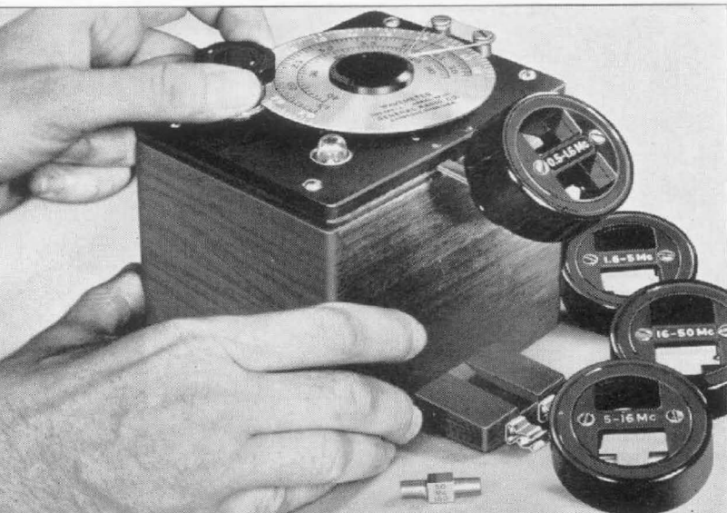
FIGURE 3. View of the TYPE 566-A Wavemeter in use. The coil can be rotated to secure optimum coupling to the source whose frequency is being measured.
