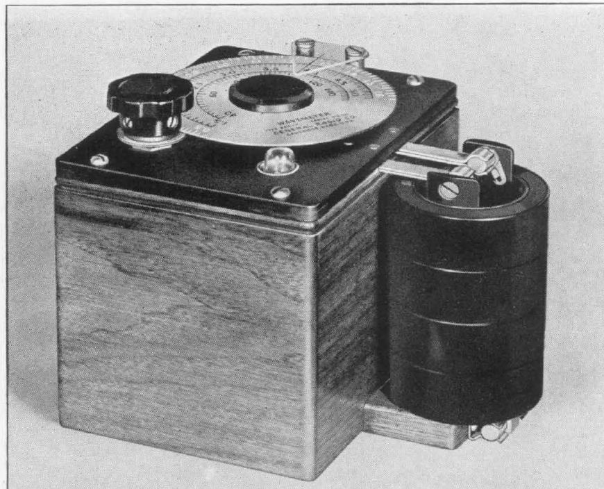
FIGURE 1. View of the TYPE 566-A Wavemeter showing how coils are stored when not in use.
