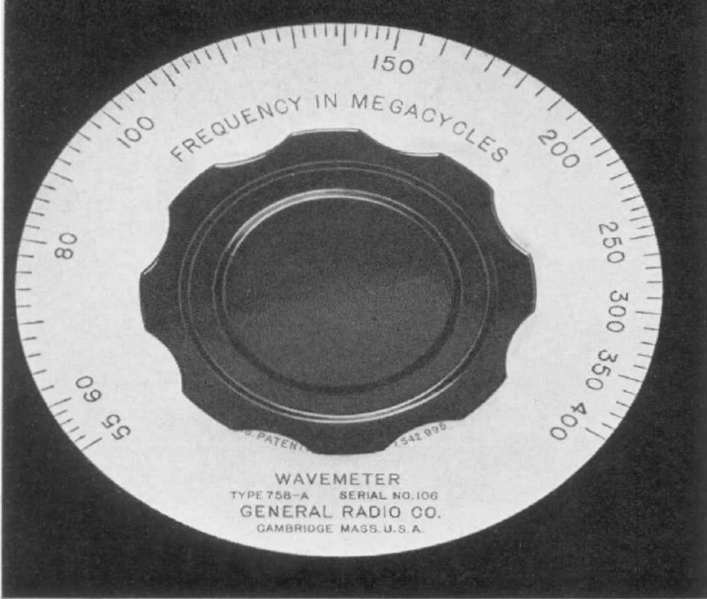
FIGURE 2. Direct-reading frequency scale of the TYPE 758-A Wavemeter.
