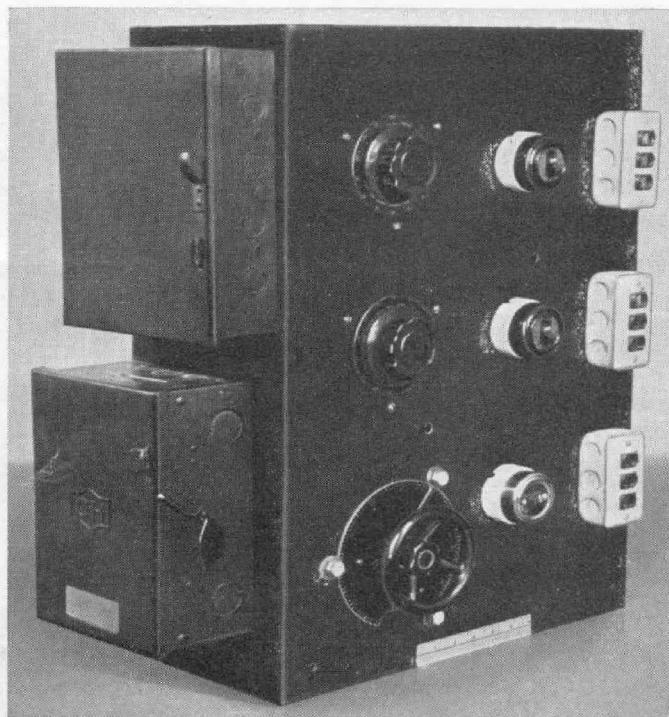
FIGURE 3. This experimental board uses one TYPE 100-K and two TYPE 200-CU Variacs. The total cost of parts for this assembly, in addition to the Variacs, was only $5.
