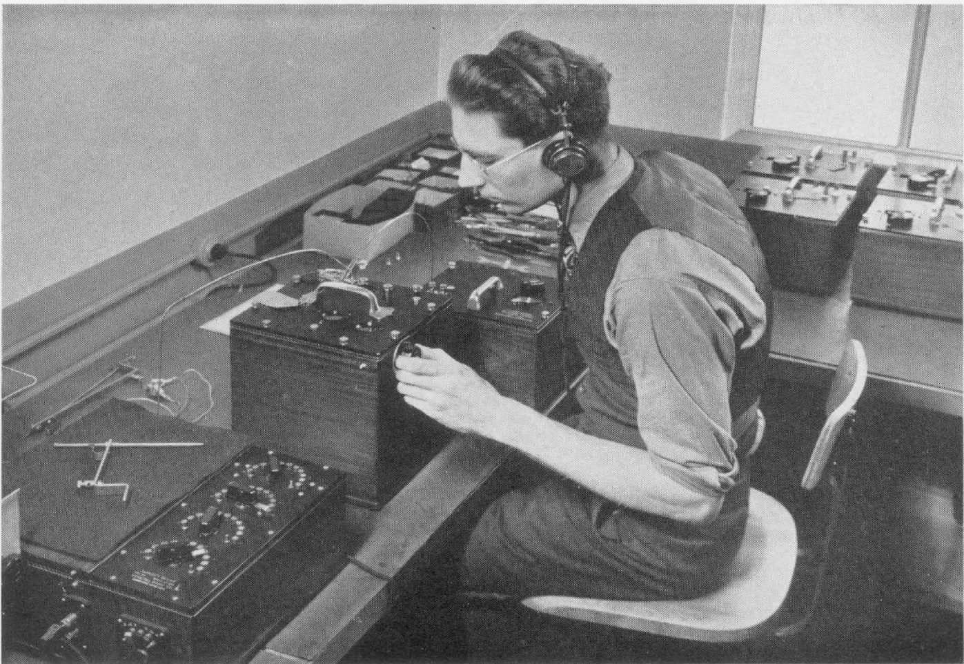
FIGURE 8. Calibrating a TYPE 722-F Precision Condenser
