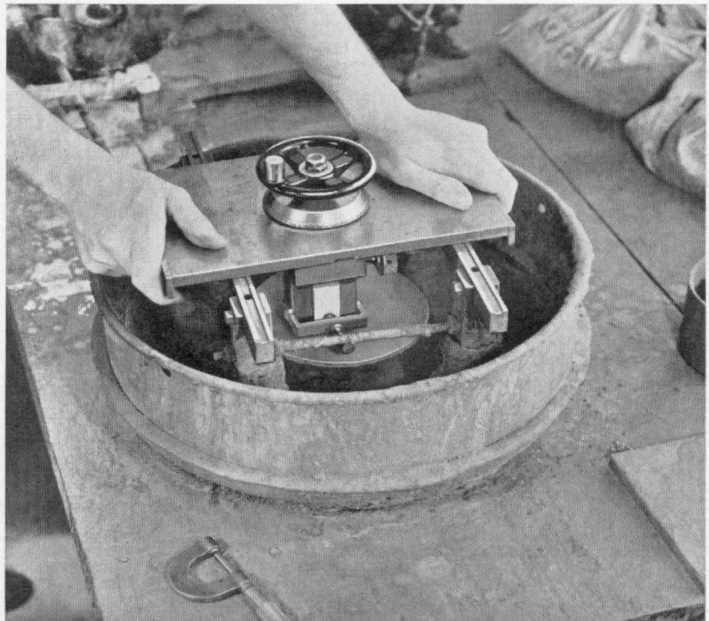
FIGURE 4. One of the grinding operations in the production of General Radio quartz plates. The edge of the plate is held against a rotating disk, and the calibrated head shows the amount ground from the edge
