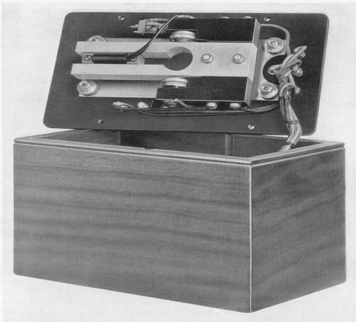
FIGURE 2. Internal view of 400-cycle oscillator, showing fork and method of mounting
