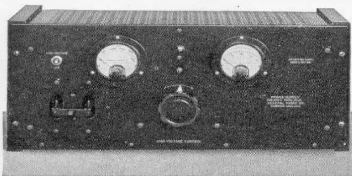
TYPE 673-A Power Supply. Practically any voltage from zero up to the rated maximum can be obtained from the high-voltage supply circuit of this unit
