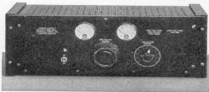
TYPE 672-A Power Supply. This is one of two new power-supply units in which the output voltage is adjustable
