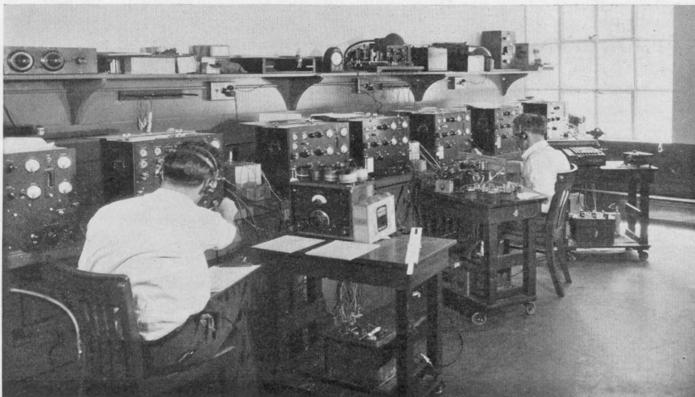
Calibrating a group of special self-checking heterodyne wavemeters designed and built by General Radio for the United States Coast Guard
