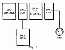
In operation, the wave analyzer is tuned to the fundamental test frequency and then to the successive harmonics to an extent determined by the amount of frequency tuning range between the fundamental and the 16 kc. limit of the dial. The harmonic amplitudes are indicated directly by the meter.
