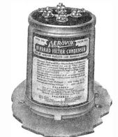
How the mounting ring is used to mount a condenser upright above a subpanel.
