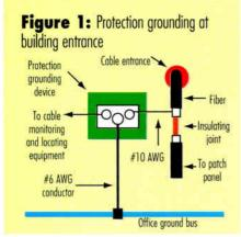
use of an "insulating joint" the outside plant cable can continue to be run into the office. This method eliminates the need for a splice enclosure at the building entrance. Local fire codes can be met by installing the cable in conduit. (See Figure 1.)
