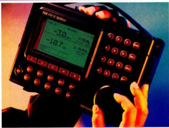
The rugged RFM150 SignalScout<sup>™</sup> signal level meter automatically performs a wide range of advanced measurements with unmatched simplicity.
