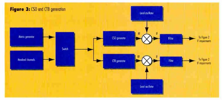
verted to a selected channel using a Gigatronics 6082A signal generator as a local oscillator with a mixer. The signal generator has very low phase noise with amplitude, frequency and phase modulation capabilities. This permits additional impairments of hum and low-frequency noise, phase noise and residual FM to be added to the system being tested.
