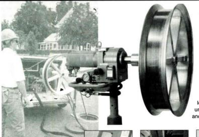
Know your flow. Only Condux offers the most accurate cable tension monitoring available... load cell torque input. It measures the actual torque at the capstan which provides a consistently true measurement of pull tension.
