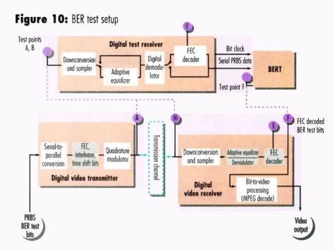
BER from the data output of the test receiver. Note that the BER reading will be different depending on whether the adaptive equalization and the FEC are applied in the test receiver. A cable operator must know what layers of processing are included in his test receiver. The test receiver may have to include an adaptive equalizer and FEC decoder for every format to be tested in the digital cable system.
