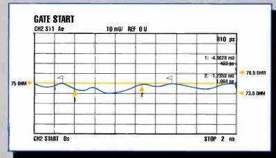
Test Procedure - Launch off 75 ohm Amphenol precision lab connector into tested connector gating out cable. Test equipment used - Hewlett Packard 8753D.
