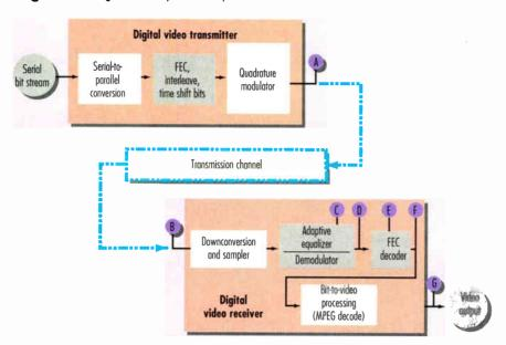
stream. FEC adds redundancy to the bit stream, making the correct data sequence recognizable even with one or more bit errors. The FEC is unique to each digital transport format. In the European 64-QAM digital video cable standard, a Reed-Solomon t=8
