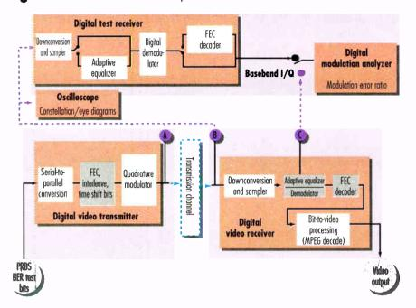
in a digital modulation format. For example, a bit stream passed into a 16-QAM modulator is first grouped into sets of four bits. Each set of four bits is a symbol, creating  $2^4 = 16$  pos-
