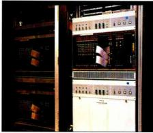
Hitachi built the multiplexer/demultiplexer used in the network.
