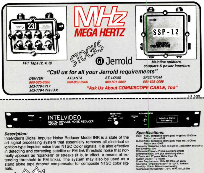
art signal processing system that essentially removes all electrical or ignition-type impulse noise from NTSC Color signals. It is also effective in detecting and correcting satellite or FM link threshold noise that normally appears as "sparkers" or streaks (it is, in effect, a means of extending threshold in FM links). The system may also be used as a stand alone tape dropout compensator for composite NTSC color sig-
