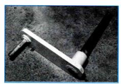
New replacement hinge pin and leveling lever arm.
