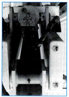
Back end of lift showing hinge pin with grease fittings and grease gun decals.
