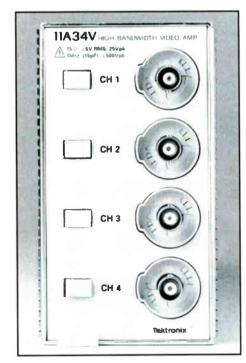
operation. The 11A34V has 75-ohm, 1 M-ohm switchable input impedance and, when used with the 11T5H, provides display clamping and trigger source signals. The unit has four 300 MHz channels, fast overdrive recovery, wide offset and dynamic range, plus a 1 mV/div. to 10 V/div. sensitivity.
