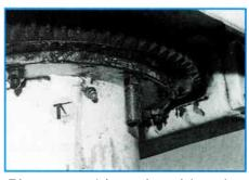
Ring gear with enclosed box for worm gear and oil bath.
