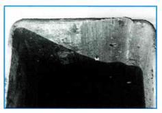
Abnormal boom wear caused by worn pads.
