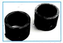
Worn bushings, rusted from lack of grease.
