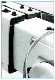
Replaceable pads on extension boom to prevent metal-to-metal contact.
