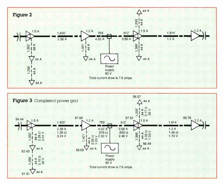
First, draw out the basic grid on paper, then write in each active device's current draw next to the active itself (Figure 1). Next, start at the most distant part of the grid and begin to add together the current draws that would be drawn through each piece of cable; write these numbers below or next to the cable itself. You'll want to work toward the power supply (Figure 2).
