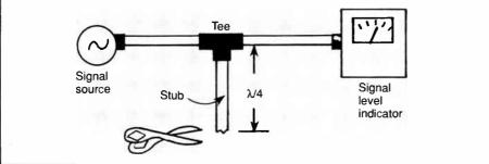
cable you use), the length of cable necessary to construct a quarter wavelength trap can be found with the following formula:
