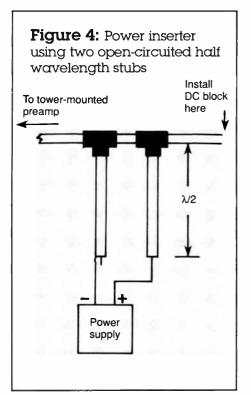
short together after each cut). As the length of the stub—which will include the connector and part of the tee—approaches an electrical quarter wavelength of the desired frequency, the offending carrier's amplitude will decrease.
