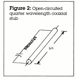
an inductor, and the open-circuited coax will take on the characteristics of a capacitor.
