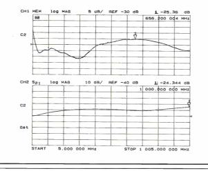
a very difficult value to measure, but all the samples tested were essentially at the noise floor of the measurement system (-120 to -130 dB). Unfortunately we could not check shielding beyond 450 MHz. In any event, compared to the stamped metal backing plate design, the Regal design is as much as 30-50 dB better.
