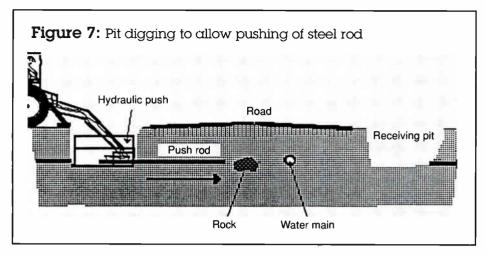
the optical cable is pulled through the duct for added protection of the cable. The metal pipes generally extend through the pit dug on each side of the road to protect the cable from added stress when the earth settles.
