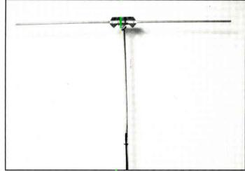
**Photo 10:** Attach the plastic bracket to a suitable wooden handle or piece of PVC pipe, tie wrap the transmission line to the handle in a couple places and install an F connector on the other end of the RG-59. The completed dipole is now ready for leakage measurements; be sure to account for the loss of the RG-59 transmission line (add it to your meter reading). In this case, the 15 feet of RG-59 has less than 0.5 dB of loss at Channel 16.
