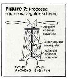
to design a dual polarized antenna with two crossed dipole feeds, then the "separator" could connect to these two feeds. The result would be one antenna for an arbitrary mix of adjacent channels (up to 31 channels). The implications at the receiving end have not been addressed.
