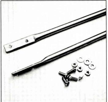
**Photo 2:** Flatten about 1¾ inches of one end of each element in a bench vise. Drill two 1/8-inch holes in each of the flattened ends, about an inch apart. Drill corresponding matching holes in each half of the plastic bracket. Select machine screws, washers and nuts of a suitable length and diameter to attach the elements to the bracket.
