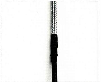
**Photo 9:** Install a small piece of heatshrink tubing over the solder connection and shrink it with a blow dryer.
