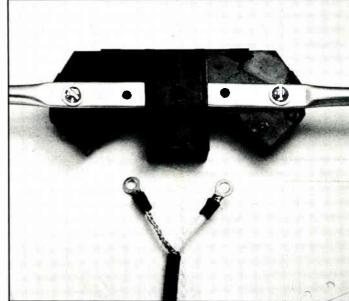
**Photo 4:** Strip back about 1½ inches of the jacket from one end of a 15-foot piece of copper-braid RG-59 cable, and separate the braid from the center conductor/dielectric. Remove about ¼ inch of dielectric to expose the center conductor, and install crimp-on automotive lug connectors on both the center conductor and shield. Solder after crimping to ensure good connections.
