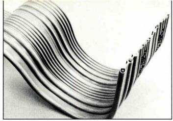
The multiple-conductor, flat ribbon cable, together with coaxial conductors, comprise the Smart House hybrid branch cable that will connect all power, control and communication services to convenience outlets throughout the home.
