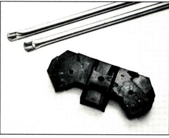
**Photo 1:** Drill out the rivets that hold one of the plastic brackets and a pair of elements to the TV antenna's boom. Use the longest elements, each of which should be about 4 feet long. The plastic bracket will be the dipole's center support, and the two TV antenna elements will be fabricated into the dipole's two elements.
