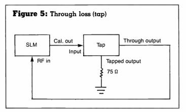
output level to the known calibrator level. During these measurements, it is important to terminate unused splitter or tap ports with a 75-ohm ( $\Omega$ ) terminator as shown in Figures 3-7.
