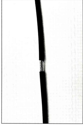
**Photo 6:** Measure 21.38 inches down the coax from the antenna (from the end of the jacket where the center conductor and shield separate). At this point, remove about <sup>3</sup>/<sub>4</sub> inch of jacket from the RG-59, being careful not to cut through the shield.
