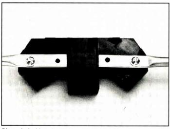
**Photo 3:** At this point, attach the elements to the plastic bracket using only the outer holes. The center holes will be for connection of the transmission line to the elements.
