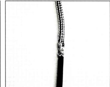
**Photo 8:** Trim the other end of the RG-8 shield to line up with the RG-59's exposed shield. After tinning the RG-59's shield, solder the RG-8 shield to it.
