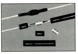
ETCON SK830, the first U.L. Listed splice kit for direct burial of UF type wire, provides reliable watertight underground connections. For use with 14gauge to 8-gauge copper wire rated up to 600V. Easy to install kit contains 4-conductor splice connector, terminal block, and required shrink tubing.
