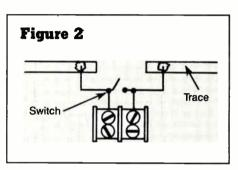
current draw but needed to figure out how to physically check it with minimal downtime. Again, I cut into the AC controlling traces on the circuit boards of an LPI and remoted these points to a terminal strip mounted on the faceplate. Then I got fancy and shunted the terminals with a switch. (See Figure 2.)
