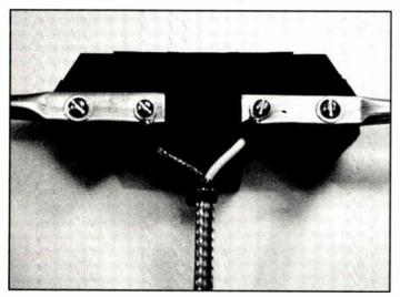
**Photo 7:** After removing a couple feet of shield from a piece of RG-8, slip that shield over the RG-59's jacket. At the top end, secure the RG-8 shield to the RG-59 with a tie-wrap. Make certain that the RG-8 shield does not come in contact with either the RG-59 shield or center conductor, but is as close as possible to the end of the RG-59's jacket.
