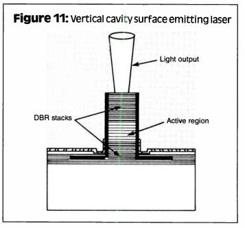
tration of light intensity at the laser's emitting facet will increase laser life and reduce risk of damage to the facet. Having lasers made with vertical emission will enable testing of the laser properties while on the wafer, in contrast to conventional lasers where each one must be mounted and tested individually. The yield of the mounting operation will increase dramatically.
