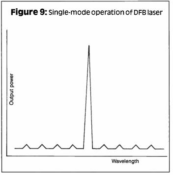
quantum wells and usually a single mode of operation is achieved, with a line width narrower than that of current DFB lasers. Another benefit of quantum well structure is a very low threshold current, enabling operation of the laser with less external electronics.
