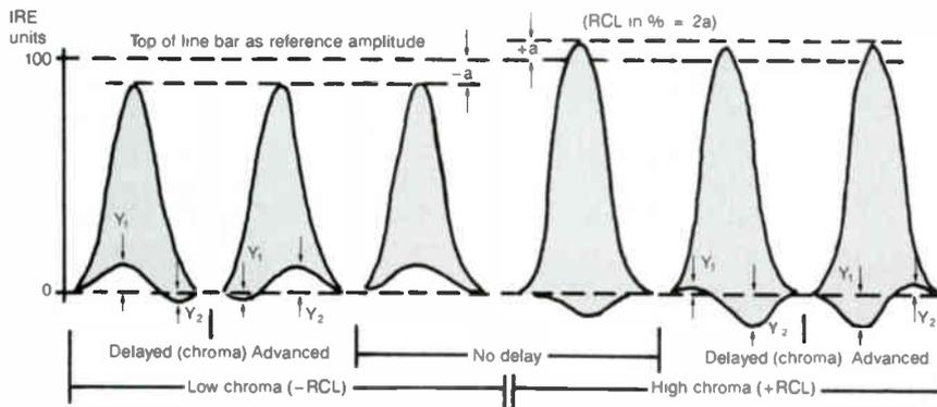
Again, we use the chrominance pulse portion of the composite test signal. The chrominance pulse is set to exactly 100 IRE (Figure 4). A starting positive going lobe should be recorded as delayed chroma. Delay inequality can be computed by CLDI (in nanoseconds) =  $20\sqrt{Y_1 \times Y_2}$  (Figure 5), or use the nomogram (Figure 6).
