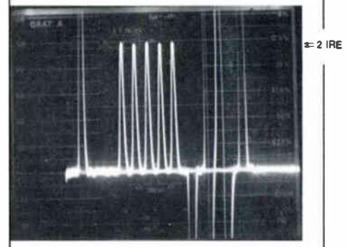
largest chroma envelope (spike) is 100 IRE. Measure the difference between the peak step and the smallest step. This is the differential gain. The parameter is not to exceed 15 IRE.
