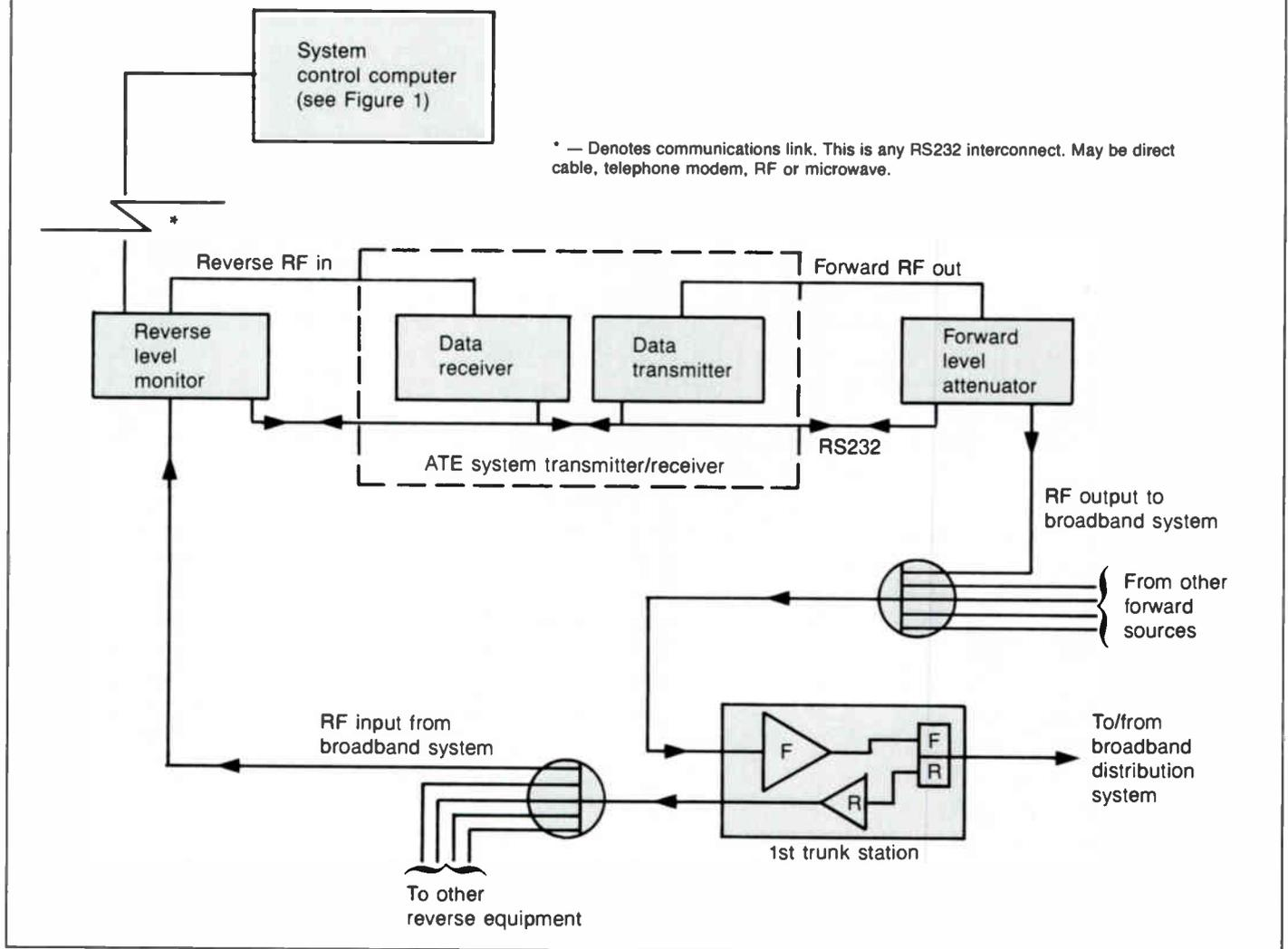
system. Figure 2 shows the headend installation. The control system can communicate with several configurations of the variety shown in Figure 2. With the basic requirements for control and communication out of the way, it is easy to understand how this system can provide tremendous functionality.
