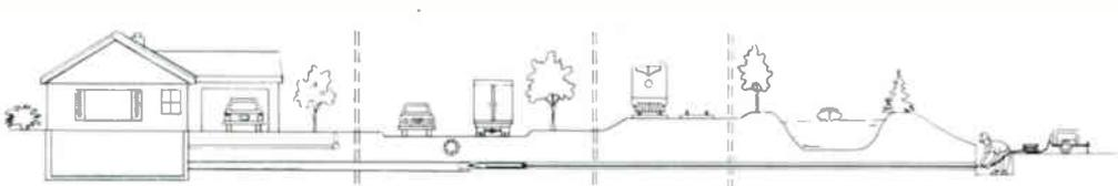
Pierce Arrow™ pneumatic underground piercing tools penetrate rocks, small boulders and tree roots, making a straight compacted hole for pipe or cable. They eliminate the added work of open trenching.
