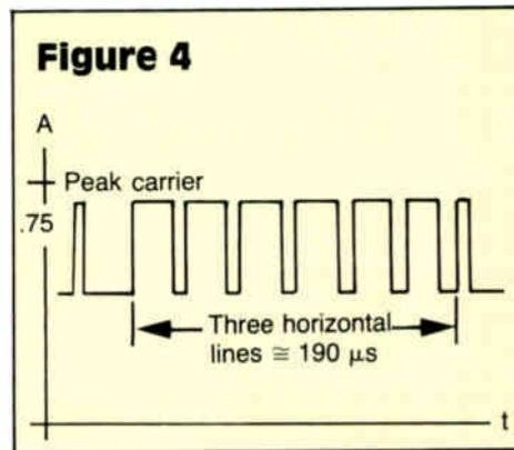
This is clearly in excess of the 160 microsecond limit. The average power of this waveform is less than peak carrier power, but it is still about 91 percent or  $-0.4$  dB, which is insignificant in our consideration. By this it should be observed that the use of average power calculations will not benefit the cable operator by allowing him to run visual carriers at higher levels.
