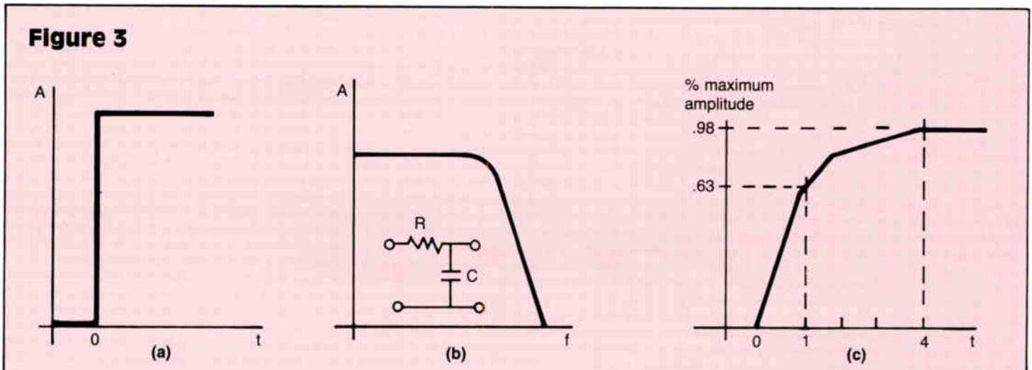
There is another effect that must be considered. When a steep wavefront, such as a leading edge of a single pulse (Figure 3a), is introduced into a narrowband filter (like a radio receiver) the output wavefront is not as steep since it takes a finite time for the signal to build up and reach its peak value within the narrow bandwidth.
