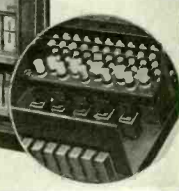
Western Electric 14-A Transmitter used at all of the land stations along the route of the Clipper ships. Note the liberal use of ISOLANTITE.
