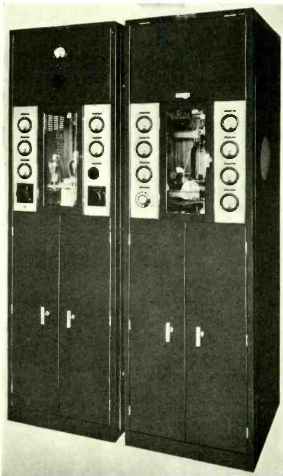
FRONT VIEW OF THE TEN-FREQUENCY RADIO QUICK-SHIFT TRANSMITTER FOR COASTAL AND OCEAN-GOING SHIPS AND AVIATION GROUND STATIONS, SHOWING THE RECTIFIER AT THE LEFT AND THE TRANSMITTER AT THE RIGHT.
