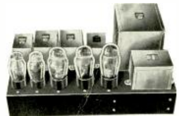
Double push-pull 2A3 amplifier using NIKLSHIELD units
