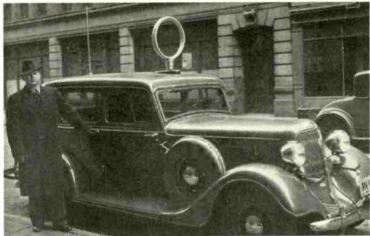
FIG. 3. INSTALLATION OF THE RADIO DIRECTION FINDER IN AN AUTOMOBILE. NOTE THE VERTICAL ANTENNA MOUNTED TO THE REAR OF THE LOOP ON TOP OF THE CAR.
