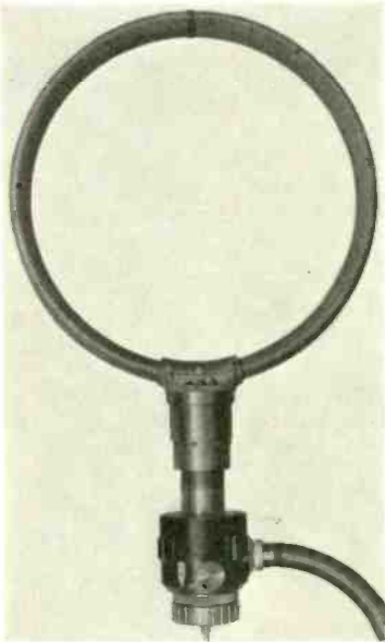
FIG. 2. THE SPECIAL LOOP ANTENNA USED WITH THE RADIO DIRECTION FINDER.
