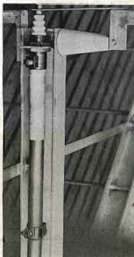
Fig. 9 (above, left) View of a dipole feed showing end terminal for a \frac{3}{8} " air-dielectric line in place.
