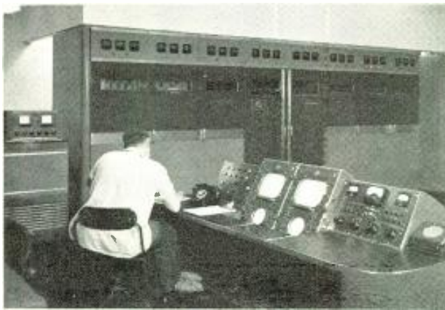
At left: WBZ-TV transmitter operating console, in foreground, with TV transmitter (background), which is located in the main equipment room. Vestigial side-band filter is at rear right. At right: FM transmitter being viewed by officials prior to the increase in power to 10 kw (left to right)—W. C. Swartley, WBZ station manager; G. W. Price, president of Westinghouse Electric, and W. H. Hauser, WBZ chief engineer.
