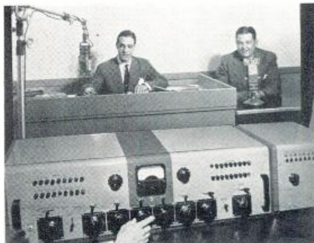
One of the two transcription studios, with announcer Carl deSuz cueing in a transcription on one of the triple turntables, while announcer Malcolm McCormack makes the station break. Studio console with channel switching unit is in foreground.
