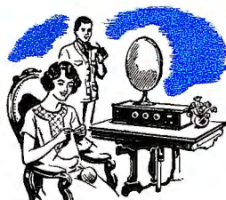
1924. Non-directional, small in size, yet extremely wide-range for its day, the 540 cone speaker designed for broadcasting was so popular for home receivers that it became a symbol of early radio.
