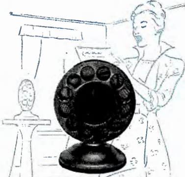
1920: Telephone scientists developed the first successful commercial mike—the double carbon button air-damped type. Used first in public address systems, it later became the early symbol of broadcasting.
