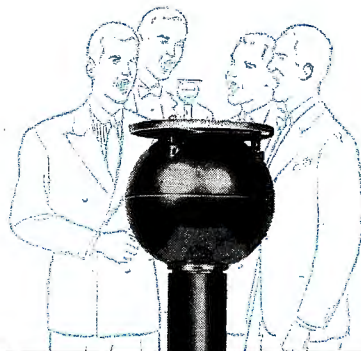
1935: The first non-directional mike — the famous Western Electric 8-Ball, designed by Bell Laboratories. Small, spherical, it provided top quality single mike pick-up of speech or music from every direction.
