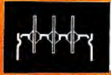
Fusite terminal panel used as cover for container. A single sealing operation.
