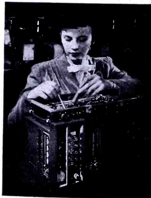
Checking a tank transmitter.
