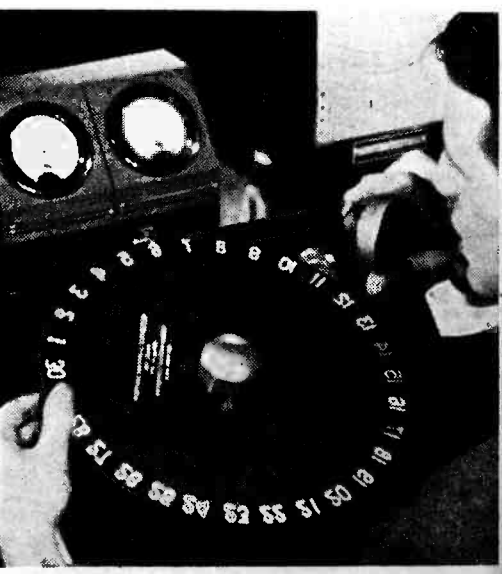
Views from the Reeves technicolor motion picture on crystals shown at the Rochester Fall Meeting. At top, blanks being placed in the holder of an Atlas lap. Below, putting crystals through a temperature run test.
