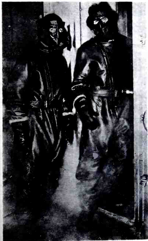
Engineers at a General Electric plant about to enter a chamber to test war radio equipment at temperatures as low as 100 degrees below zero. The cold surpasses that encountered by Arctic-bound ships or planes flying in high altitudes.
