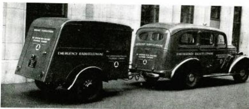
Figure 2 Trailer with transmitter-receiver unit. The transmitter-receiver is located on a 90° rotating hanger at the left of the entrance door. This arrangement provides for easy access for operation and repair. Incoming wire lines terminate on protectors mounted on the wall.
