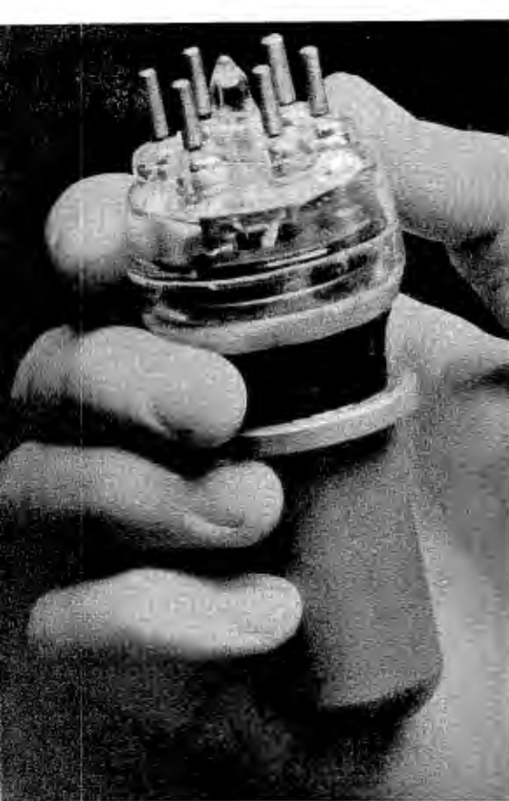
Figure 1 A water-cooled transmitting tube that is used in ultra-high-frequency broadcast service.
