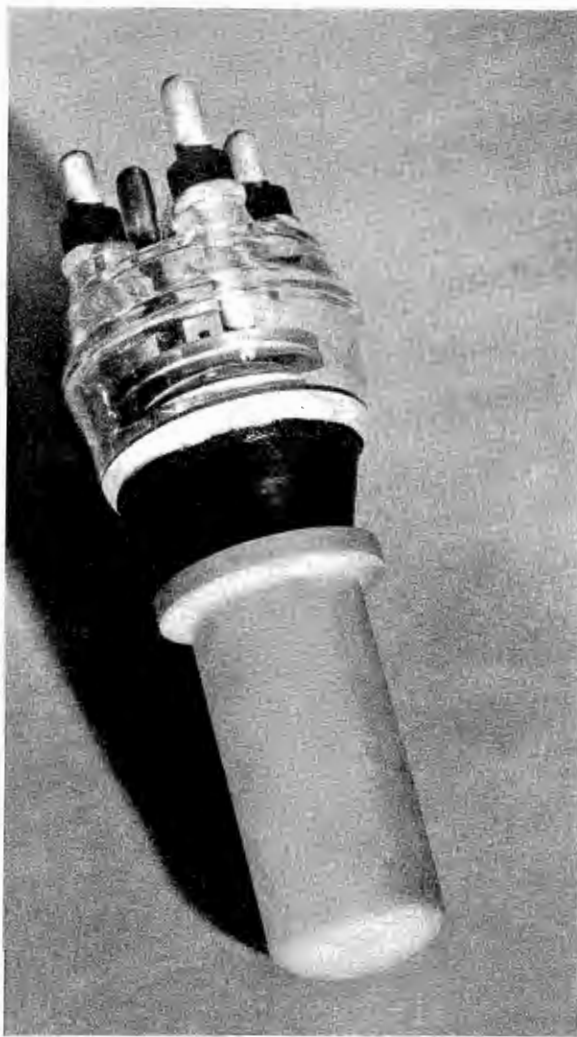
Figure 2 A triode transmitting tube, the 889, that uses a water jacket for cooling. This tube is used in the r-f power amplifier or as a class B modulator for high frequency broadcast service. Its plate dissipation is 5000 watts.
