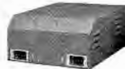
Bendix combination transmitter and receiver with two Cannon Connectors for rack use.
