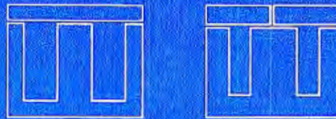
BLANKED LAMINATION TO SCRAPLESS SAVING 35% SILICON STEEL
