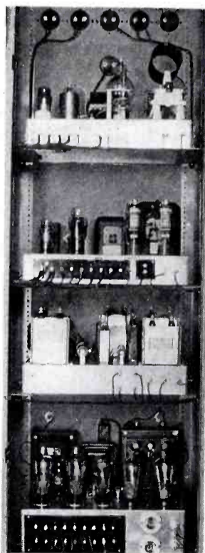
Rear view of a 100 watt transmitter used in the district dams. This unit was designed and built by the author.
