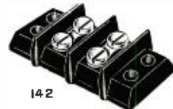
142 1-5/16" wide by \frac{3}{8} " high. 2 to 17 terminals. 8-32 by 5/16" screws.
