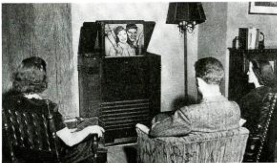
The large screen home television receiver. This instrument has a 13½ by 18 inch retractable screen which slides down into the cabinet when the set is not in use. Projection is from a 5-inch kinescope, the size of the picture on this tube being 2¼ by 3⅜ inches.
