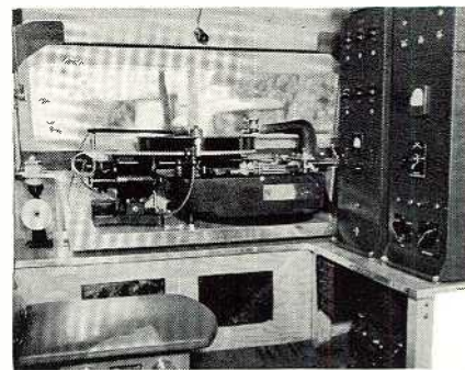
An inside view of the truck showing the professional recorder and associated equipment. Remote amplifier is also furnished.
