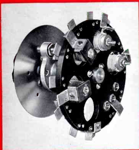
Coil assembly mounted on mycellex disc attached to switch system. Polystyrene coil insulation with unwound plug-in coil form for any additional frequency range desired; excellent electrical contact between silver-plated switch blades and contact springs.
