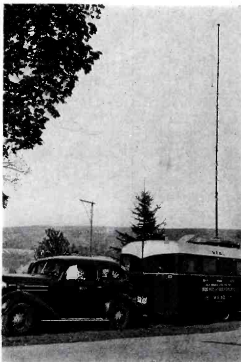
Showing the 35-foot telescopic antenna in operation at a fixed location. The lead-in is permanent, being sufficiently flexible to allow raising and lowering antenna.
