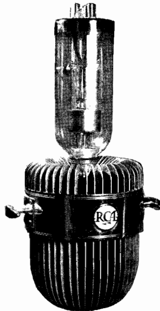
Fig. 2. One of the standard metal-anode type tubes fitted with copper radiating fins for air cooling.
