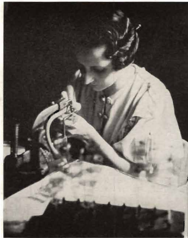
Experienced artisans spot-weld the various parts together to form the assembly which is sealed into the glass envelope of a tube.
