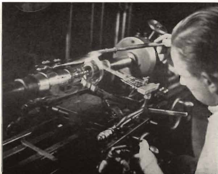
The copper-to-glass seal of a water-cooled type transmitting tube is made by mounting the tube in a device similar to a lathe. As the tube rotates, the gas-flame "tool" unites the materials.
