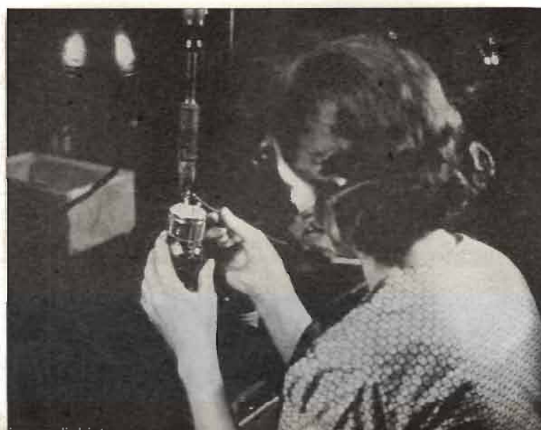
The heavy soldering copper is suspended so that the operator may hold the comparatively light vacuum tube up to it in the process of soldering the leads into the base pins.
