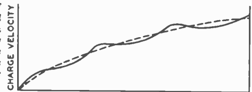
Fig. 3—Accompanying the decreasing electron densities graphed in Figure 2 are increasing electron velocities. The analogous sound wave would be one taking place in a wind whose velocity increased as it passed from cathode to anode
