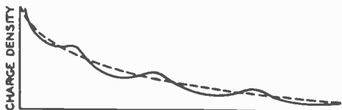
Fig. 2 (Left)—A graph of the electron densities pictured in Figure 1 shows them falling off in passing from the cathode to the anode
